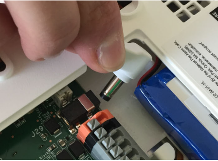
Plug in the power connector
