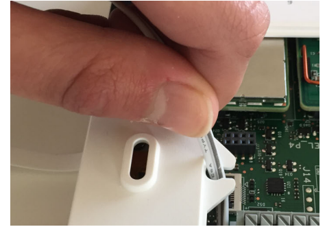
Insert the wire into the strain-relief
