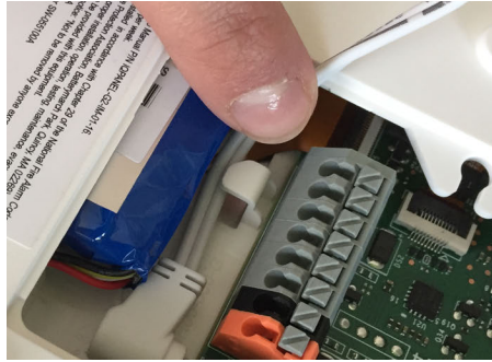
Route the wire behind the retainer clip
